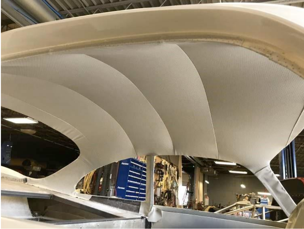
German perforated headliner being stretched into P1
