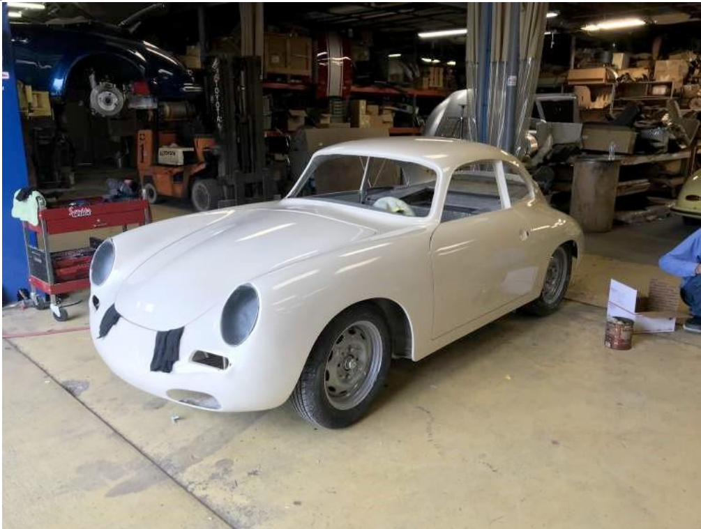
Fresh out of paint and hanging panels before trim
