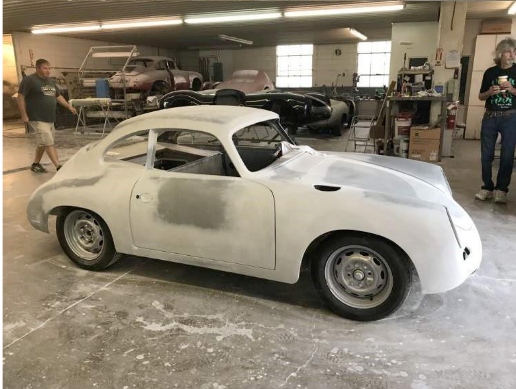
Final body work just prior to paint
